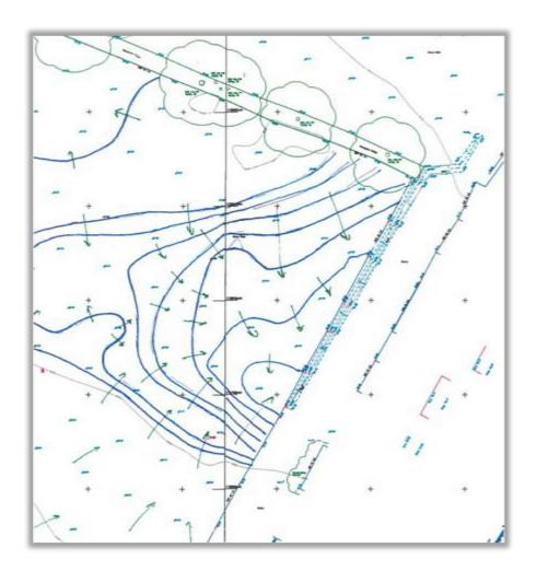
This low spot appears to be the recipient of a larger contributing area of the southern field. Local representation and photographic evidence supports this situation showing water accumulating here.
