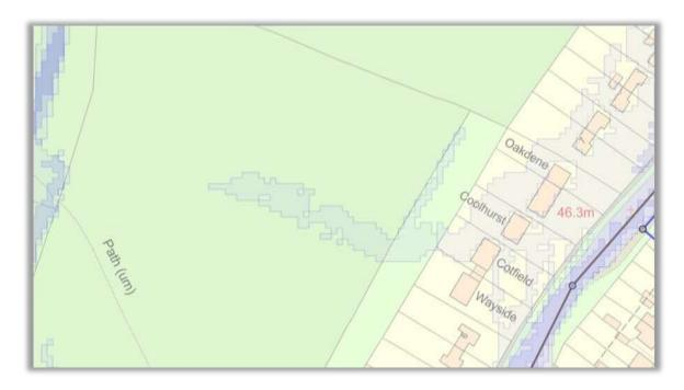
The site generally falls from South to North. But along the east boundary of the southern field, ground levels fall to the east, supporting the suggested flow route shown in the surface water flood maps. When taking the topographical survey and applying approximate contour increments of 0.1m the following is found:
